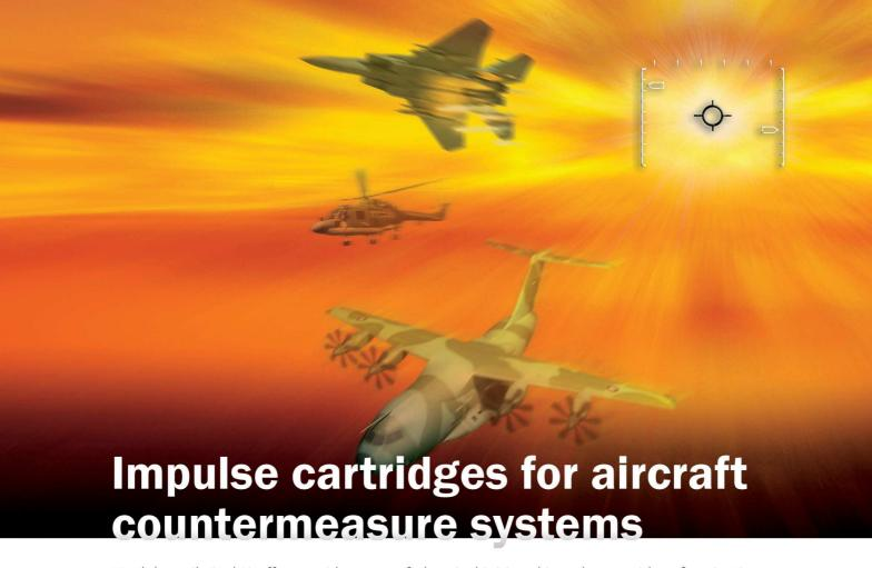
PL Elektronik GmbH offers a wide range of electrical initiated impulse cartridges for ejection of IR decoy flares against IR missiles as well as ejection of chaff against RF missiles installed on military combat jets, transport aircrafts, helicopters, vehicles and naval vessels.
