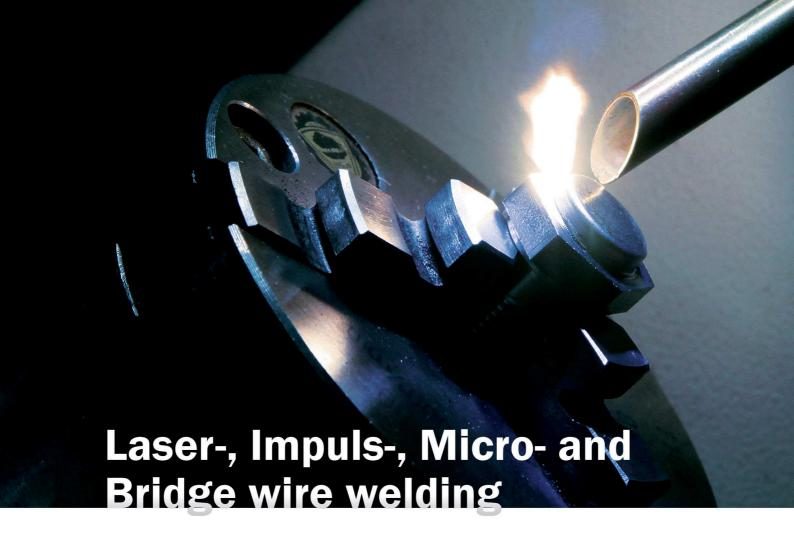
The laser, impulse and micro welding are an important key for the functionality of our products. Due to our long experience we are able support our customers in this field and can also offer the laser, micro and bridge wire welding as service for external customers. For the processing of your orders a modern TRUMPF Laser-Station is available for example.
